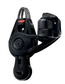
Fiddle sheave has a high load full contact bearing (ie. not ball bearing). Main sheave has two-stage, ball bearing.
