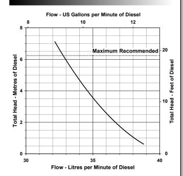
**Current Draw** 12V = 15 Amps @ 3m head 24V = 7 Amps @ 3m head
